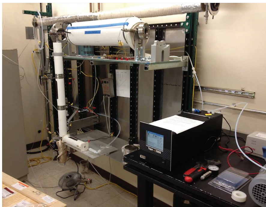
Figure 3. EPRI test set-up at UC Riverside; Tiger-i analyzer, with sample pump and Teflon® line connected to sampling manifold (sample cell upper left)
